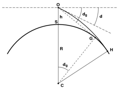
The solid arc OH now represents the curved line of sight; H is the (refracted) apparent horizon. Notice that refraction lets us see a little farther, if the ray is concave toward the Earth, as shown here.
