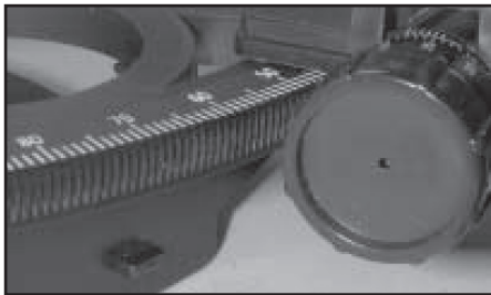
Figure 1-4 Top Close up of the worm gear on a metal sextant. A similar mechanism is encased in plastic in the Mark 15. When the clamp is compressed it pulls the worm gear out of the notches in the arc.
