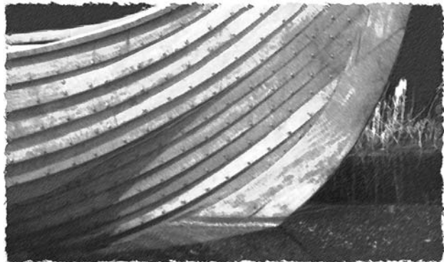
We chose pine planking for lightness and flexibility for the hull.
