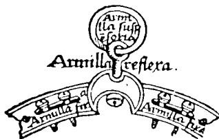
Suspension apparatus of a western astrolabe, from J. Koebel: Astrolabii Declaratio 1532.
