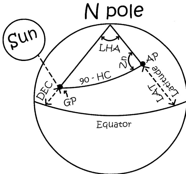
Figure one is the familiar Nautical Triangle showing the latitude (Lat) of the observer at the assumed position (AP), the declination (Dec) of the ground position (GP) of the celestial body, and the Local Hour Angle (LHA) between the GP and the observer. The  $LHA = GHA - Longitude$  (West longitude considered positive, East negative, in this convention). Then the calculated altitude (HC) and meridian angle (Z) of the body is given by the standard formulas of spherical trigonometry:
