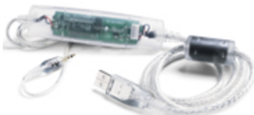
USB cable connects TI-89 to PC. CD included.
