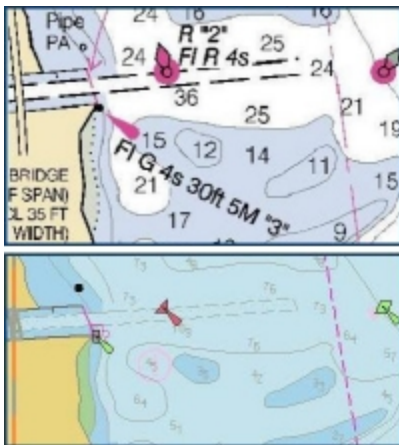
Section of RNC (top) and ENC (bottom)
