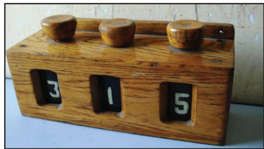
Figure 3. Course boxes were a traditional way to keep the present course posted for all to see in the cockpit or wheelhouse. Some equivalent remains an asset to navigation on all vessels. Periodically these become available online from decommissioned vessels or antique sellers.
