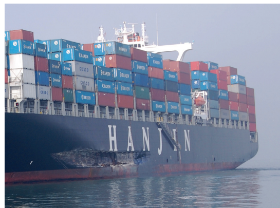
Figure 2. The damaged MV Cosco Busan after striking the bridge tower fender. There was a professional pilot on board who is tested on local knowledge to get the license. He also tested positive for a lot of other things after the allision with the bridge.
