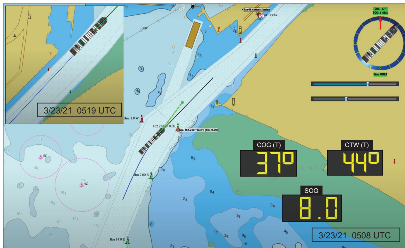
Figure A7-1. Screen capture of a video reenactment of the grounding of the Ever Given in the Suez Canal based on AIS data that include both heading (CTW, black line) and COG (green line). The look ahead time (green dot) was 2 minutes. A strong southerly wind pushed the boat to the left (green line left of the black line). The meters tell us the drift was 7° at this time, 0508. The correction to the right was not adequate to keep the vessel off the left bank, and 11 min later, about 1.5 nmi to the north, it came close enough to the bank that hydrodynamic effects almost certainly affected its motion (insert). The center section is dredged to 25m; from the dotted line to the buoys the bottom slopes from 25 m to 11m; the draft of the ship is 16m. The reenactment, showing these navigation data as the vessel progressed to the point of grounding, can be seen at starpath.com/evergiven , which includes several background videos. The grounding took place on the right bank at 0543 after a close encounter on the right, then again on the left.
