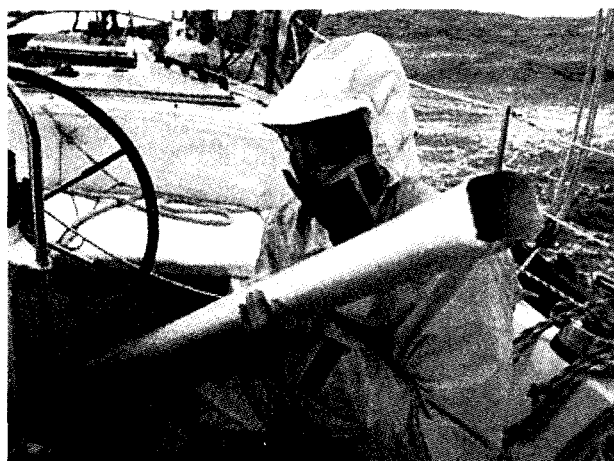
Bob inspects the breaks in the whisker pole.
