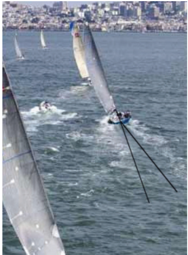
Figure 1. Sailboat wakes... not really showing much! The two left are essentially straight aft. It is light air and they are both cracked off the wind, so we would expect them to be straight. If we were to detect any leeway visually, they would have to be closer to the wind and the wind stronger. In that case, the two lines shown would be leaning somewhat off to the left, upwind. We might still see a few degrees in the ECS track however, even when not at all visible by eye.
